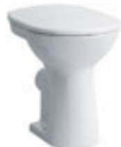
H825955 Floorstanding WC ,comfort', washdown, with flushing rim, outlet horizontal, sitting height 450 mm (without WC seat)
