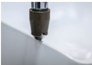
THE THIN-WALLED SAPHIRKERAMIK WAS TESTED FOR IMPACT RESISTANCE AT THE KERAMIK INSTITUT MEISSEN
